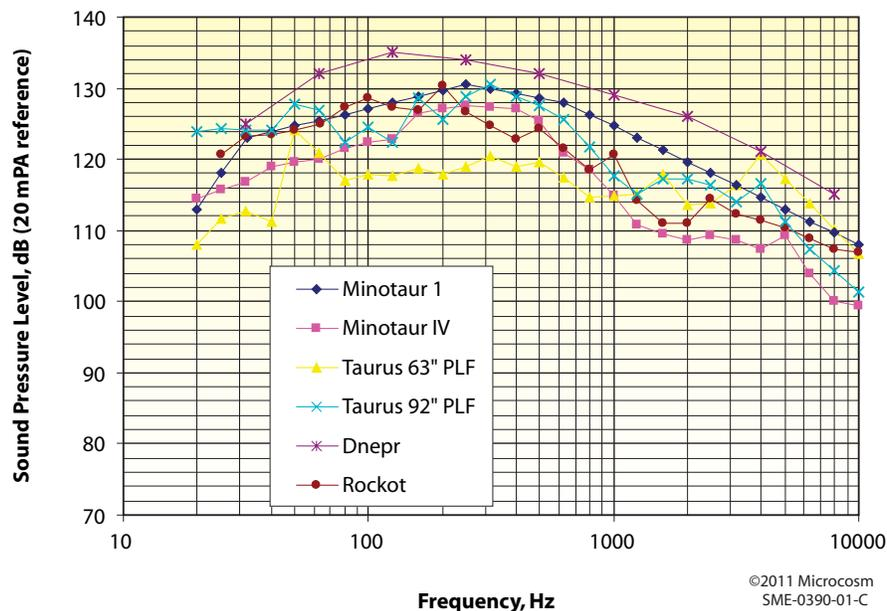
Fig. 26web-2. Example Vehicle Acoustic Environments [OSC, 2006a; OSC, 2006b; OSC, 2010b; ISC Kosmotras, 2001; Eurockot, 2004].
