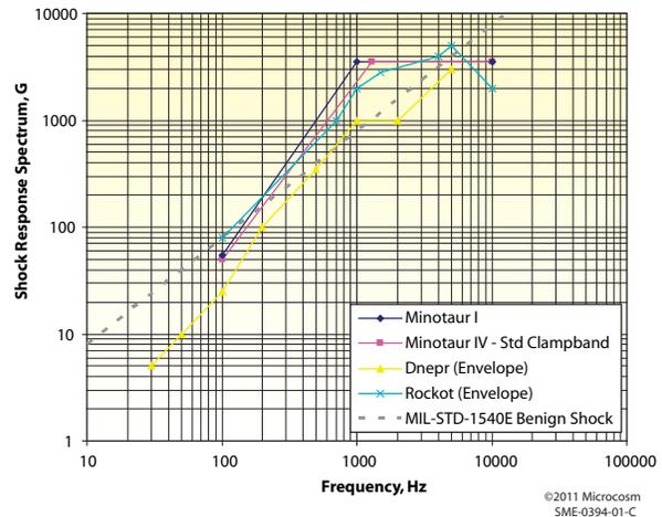
Fig. 26web-1. Example SRS for Four Launch Vehicles [OSC, 2006A; OSC, 2006b; ISC Kosmotras, 2001; Eurockot, 2004].
