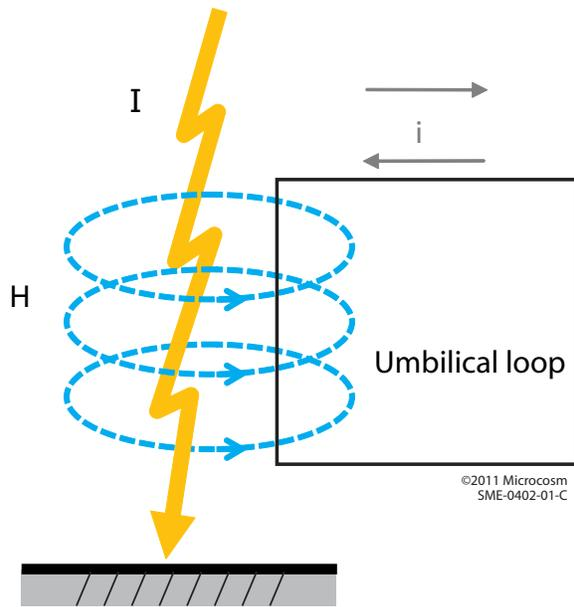
Fig. 26web-3. Lightning-Induced Magnetic Field Coupling Effect.
