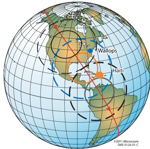
Fig. 10web-2. Motion of the Spacecraft Along the Orbit Showing Visibility Regions for Both Haiti (Solid Circle) and Wallops Island (Dashed Circle).
