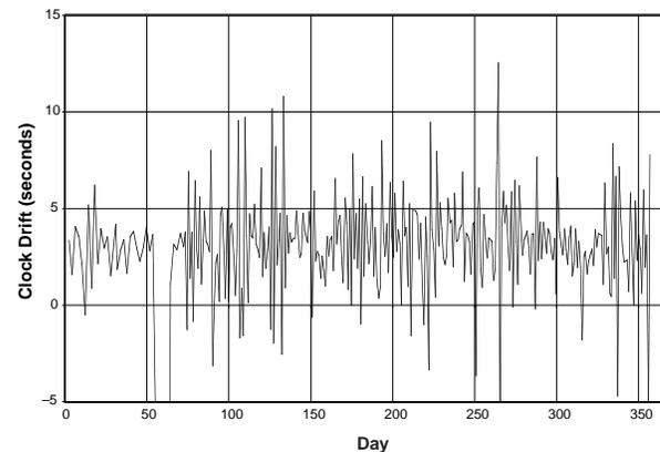
**Fig. Eweb-2. Day-to-Day Difference Between GPS Clock and BREM-SAT Computer Clock.** The figure shows fine drift of the BREM-SAT computer clock vs. a GPS clock on the ground. The results are for each day, not cumulative.
