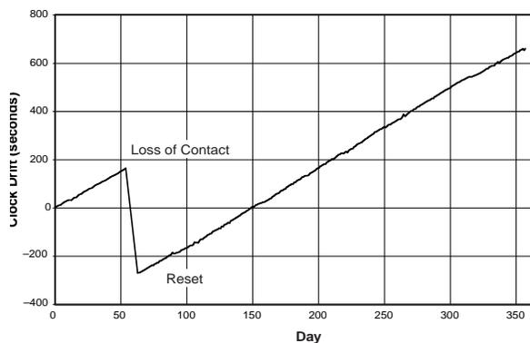
**Fig. Eweb-1. Difference Between GPS Clock and BREM-SAT Computer Clock.** This figure shows the cumulative large-scale drift of the BREM-SAT computer clock vs. a GPS clock over a year. The sharp drop shortly after day 50 reflects the loss of contact with BREM-SAT and subsequent reset after reacquisition.
